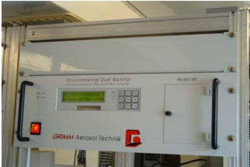
The slide bars provided by the customer for the 19" drawer have to be mounted. Subsequently mount the EDM180 and connect it to the power cable. The power cable has to be provided by the customer
