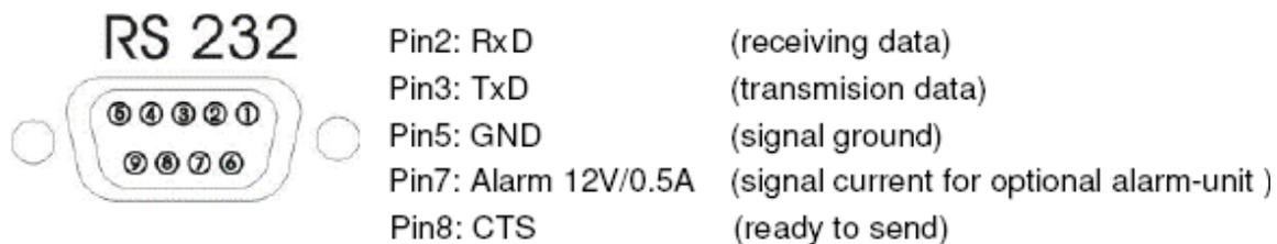
Figure 4: Pin alignment of the socket at the dust monitor „RS-232 to PC“
